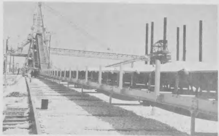
The 660-ft. yard belt of sulfur stacker. Faha di 660 pia largo pa transporta azufre.
